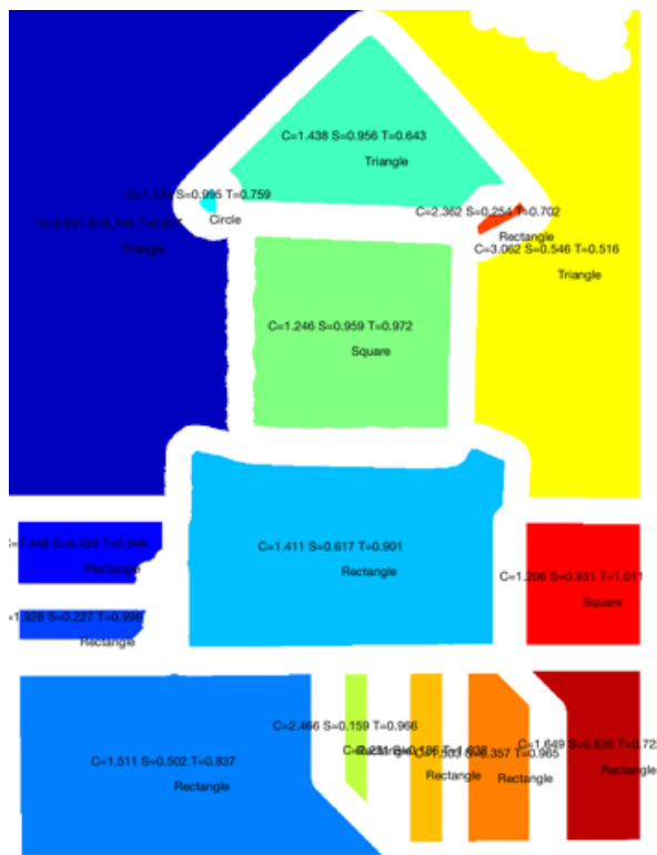
Fig. 12. The additional artefacts and the components of interest identified by the RBC algorithm.
