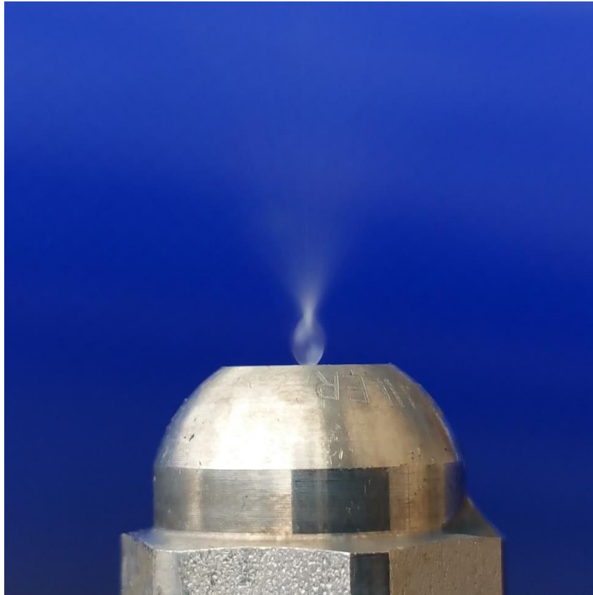
Figure 6-3 – 0.6mm hollow-cone nozzle at 4ml/min
