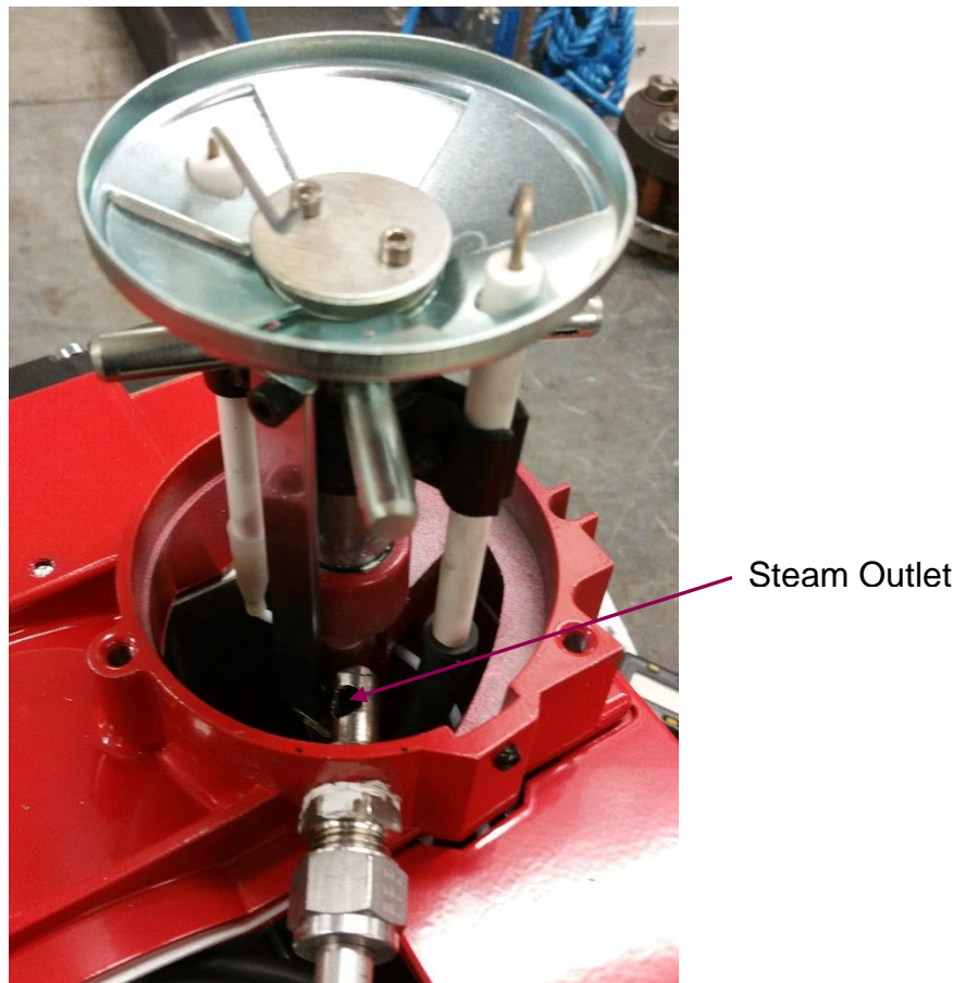
Figure 7-1 - Burner modification for steam input
