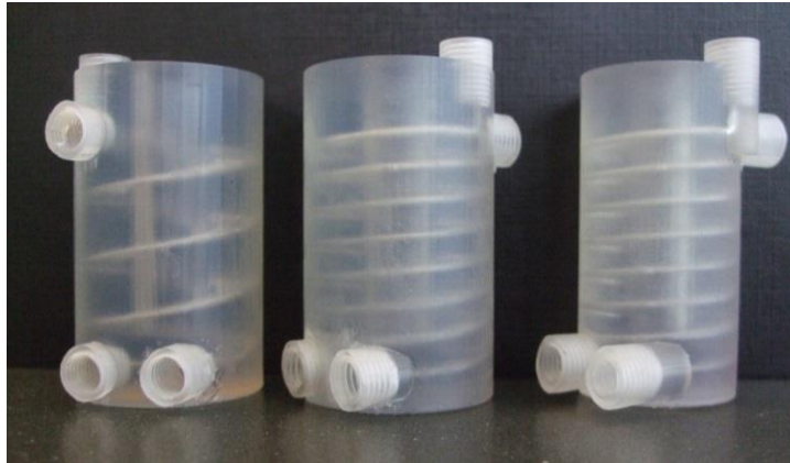
Figure 6.12 Photographs of three printed spiral magnetic separators printed via SLA in Accura® 60 polymer, each comprising of a central magnet cavity surrounded by two parallel, bridged microfluidic channels. Left to right: a) bridges: 6, pitch: 10.0 mm, shielding polymer thickness: 3.0 mm, and air gap: 1.0 mm, turns: 4, b) bridges: 12, pitch: 7.0 mm, shielding polymer thickness: 3.0 mm, turns: 7, c) bridges: 12, pitch: 5.0 mm, shielding polymer thickness: 2.0 mm, turns: 7.
