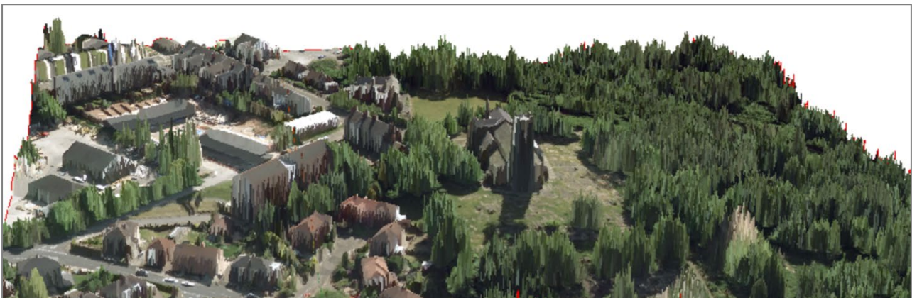
Figure 12: St Mary's Church and surroundings, Prestwich, Manchester. 25 cm LiDAR data draped with aerial photo (date flown 11 June 2015, time unknown)
