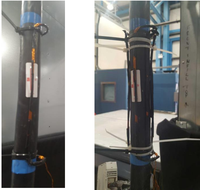
Fig. 5. Photo of a single coil and multiple coils to detect magnetic field
