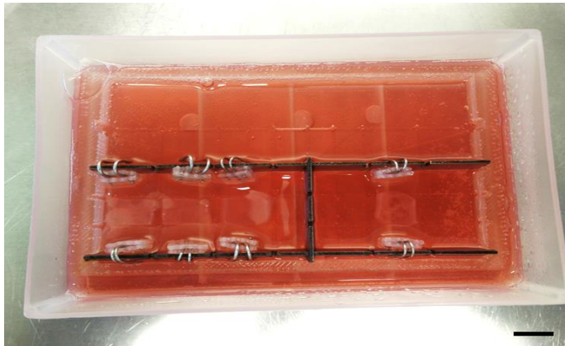
Figure 3.13: Image showing PDMS mould method with segmented gels (unseeded- C_2C_{12} – unseeded) at day 4. Gels showed little contraction with regions of adhesion between the gels and the mould. Scale bar = 10 mm
