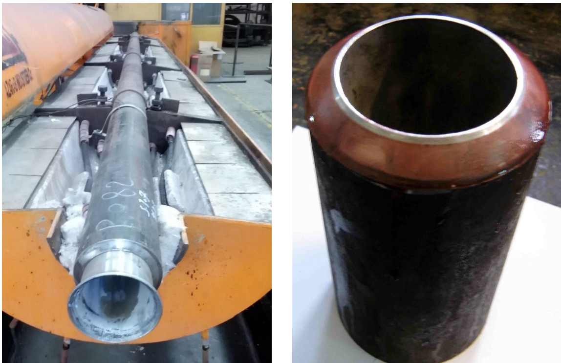
Figure 2: Experimental setup of THSF process (left); lined pipe produced for this study (right)
