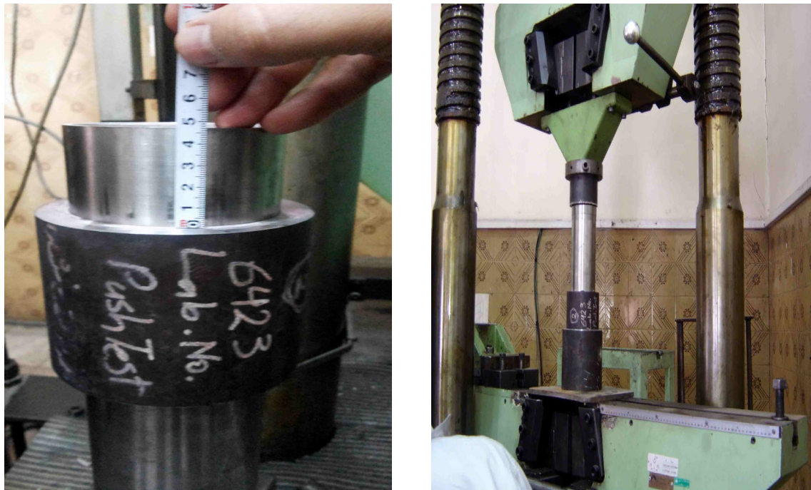
Figure 3: Experimental setup for push-out test (left); sample after pushing out inner pipe (right)
