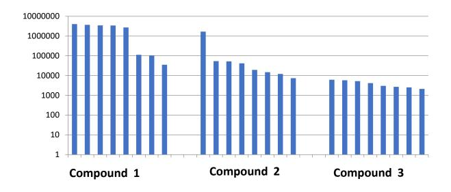
Fig 1 - Flex life of the silica-filled rubber vulcanisates
