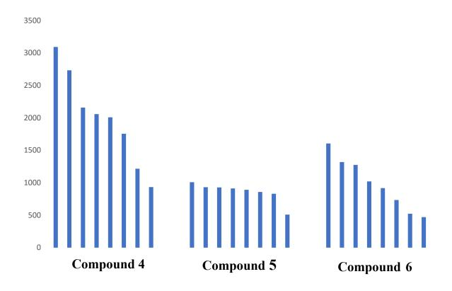
Figure 2 – Flex life of the unfilled rubber vulcanisates
