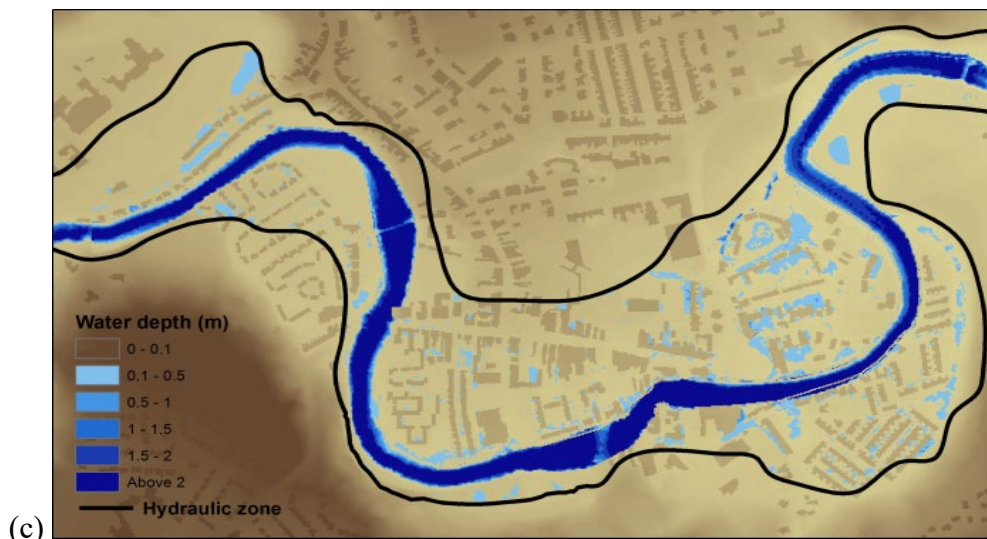
Figure 10 Inundation maps at 11am in the town centre: (a) post-event investigation (Parkin, 2010); (b) full 2D model; (c) coupled model.
