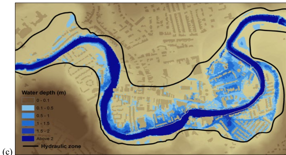
Figure 12 Inundation maps at 3pm in the town centre: (a) post-event investigation (Parkin, 2010); (b) full 2D model; (c) coupled model.
