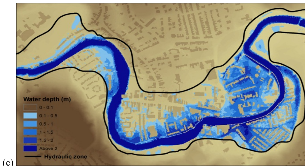
Figure 13 Inundation maps at 5pm in the town centre: (a) post-event investigation (Parkin, 2010); (b) full 2D model; (c) coupled model.
