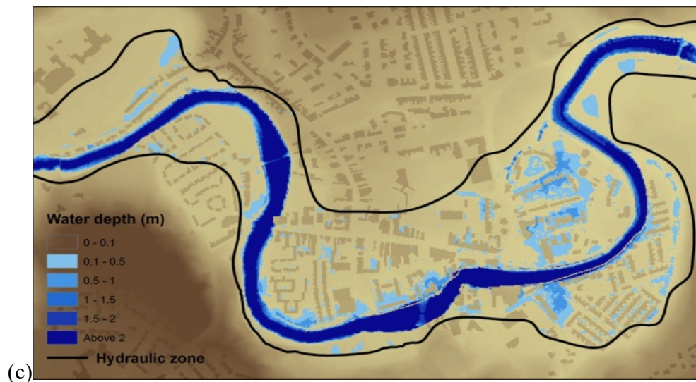
Figure 11 Inundation maps at 1pm in the town centre: (a) post-event investigation (Parkin, 2010); (b) full 2D model; (c) coupled model.
