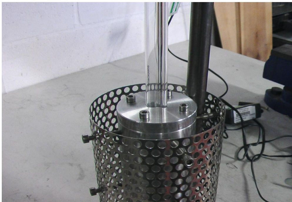
Figure 3.8 Photograph of the chemisorption apparatus to quantify acidic sites in the catalyst.
