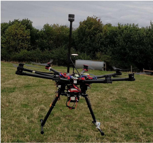
FIGURE 4 S1000 multirotor unmanned aerial vehicle with FT205EV ultrasonic wind speed sensor mounted out of rotor wash used to perform the wind field measurements [Color figure can be viewed at wileyonlinelibrary.com ]
