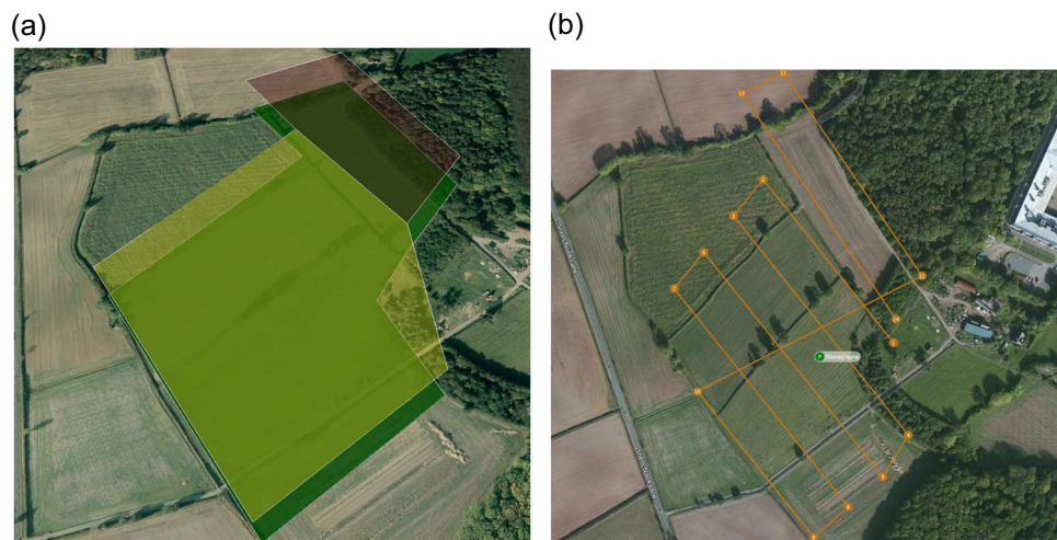
FIGURE 19 Google maps images of decomposition and way-points used for accuracy assessment surveys (a) field polygon and its RGS FTIW decomposition and (b) CPP way-points generated, to be uploaded to autopilot. CPP, coverage path planning; FTIW, flight time in wind; RGS, recursive greedy search [Color figure can be viewed at wileyonlinelibrary.com ]
