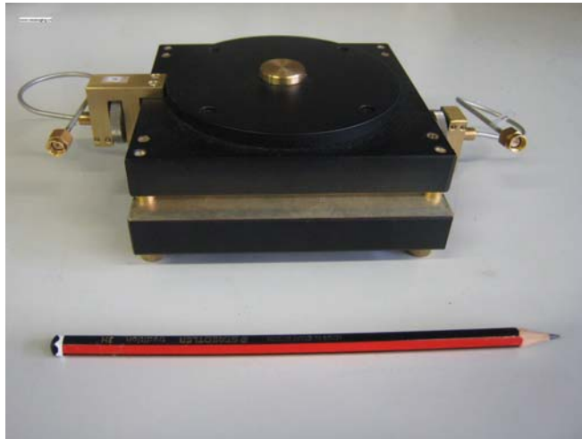
Figure 3-3 Front view of 2.4GHz Split Post Dielectric Resonator
