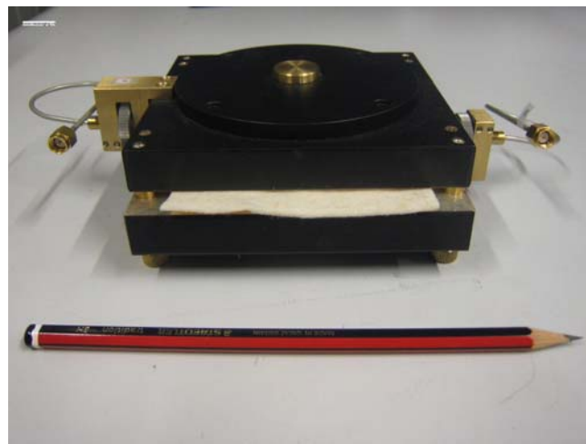
Figure 3-5 2.4GHz Split Post Dielectric Resonator with Felt sample
