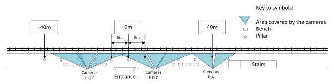
Figure 3 - Platform diagram and positioning of the video cameras
