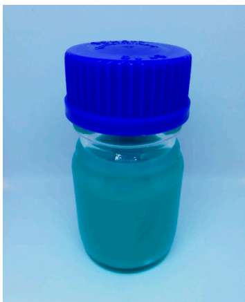
Figure A1. A mixture of 1.6 g \text{Cu}(\text{OAc})_2 \cdot \text{H}_2\text{O} and 1.5 g OH-mBDC in 100 mL DMSO after 2 h, showing a precipitation occurred in [\text{Cu}_{24}(\text{OH-mBDC})_{24}]_n stock solution.
