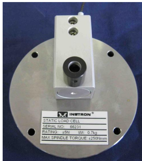
Figure 5.4. Instron 2530-436 load cell ( \pm 5 N) used for single fibre testing
