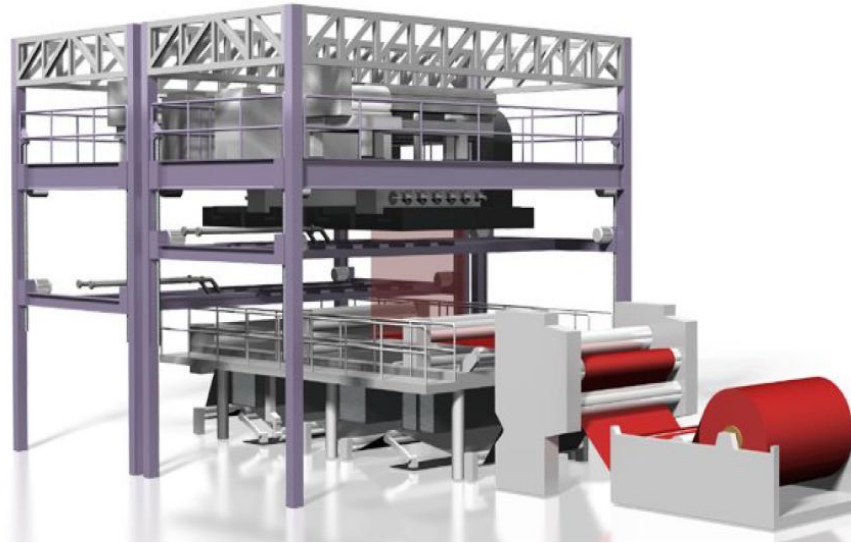
Figure 2.2. Nonwoven production facility (Hietel, 2006)
