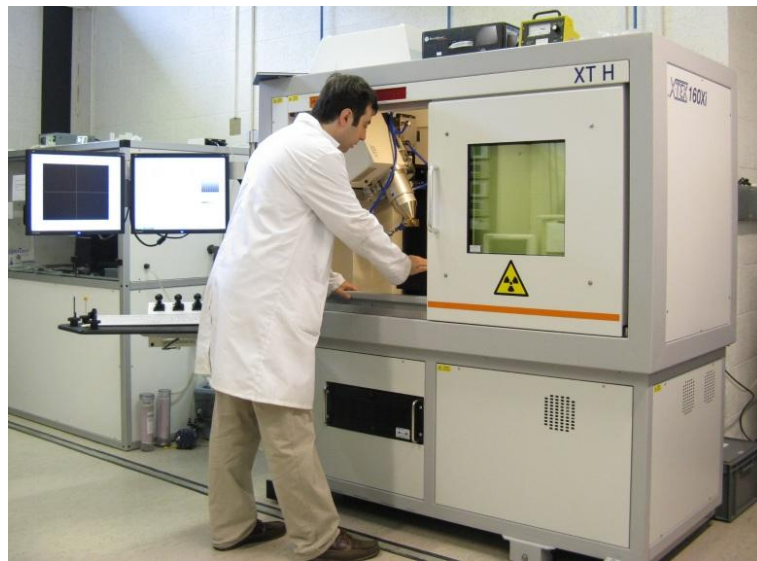
Figure 5.17. X-ray micro computed tomography device, Loughborough University, UK
