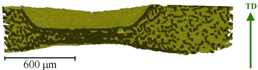
Figure 5.27. X-ray micro CT image of through-thickness cross section of thermally bonded nonwoven (fibre: PA6/PE, planar density: 150 g/m 2 )
