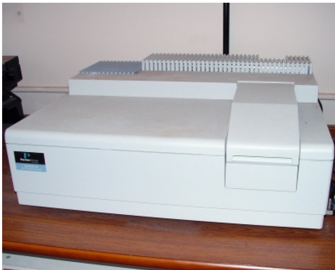
Figure 37 A Perkin Elmer Lambda 35 bench-top UV-Vis Spectrophotometer located in the Chemistry department, Loughborough University [213]
