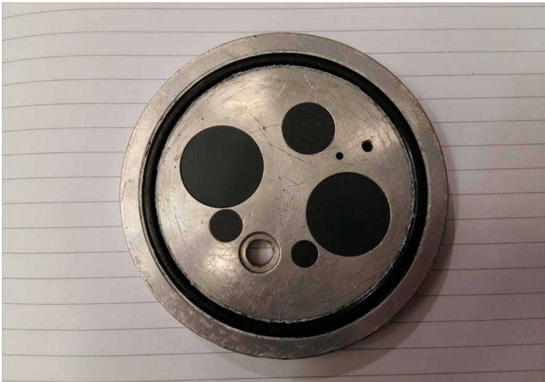
Figure 41 (a) the gas gun of the SHPB [217] and (b) the aperture plate used to control the SHPB projectile velocity
