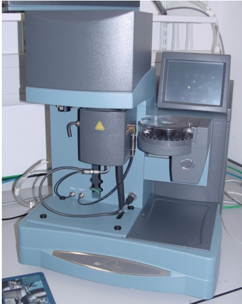
Figure 32 TGA located in the LMCC, Materials department, Loughborough University [203]
