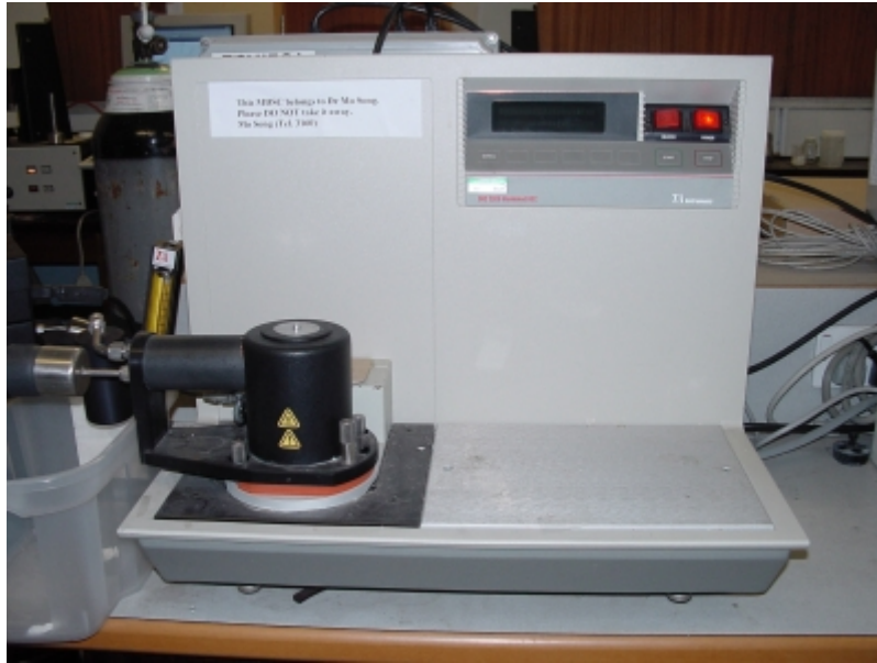
Figure 34 Modulated DSC located in the Materials department, Loughborough University [203]
