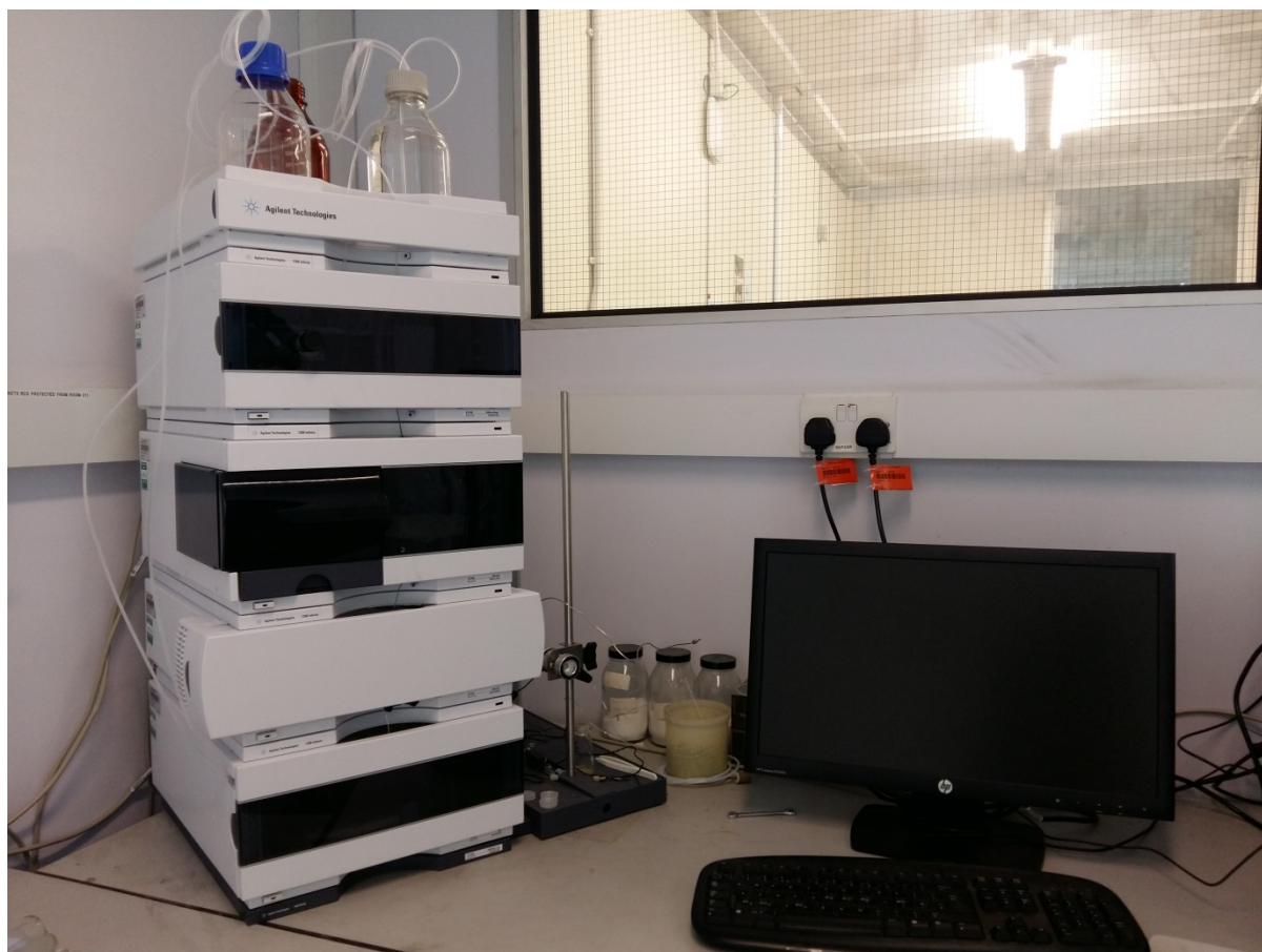
Figure 31 Agilent Technologies 1260 Infinity GPC located in the Materials department, Loughborough University
