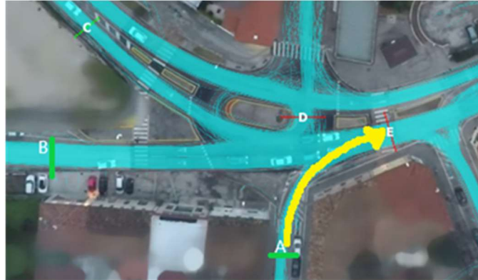
Figure 10. The vehicle trajectories marked in light blue and target maneuver shown in yellow for Italy dataset.
