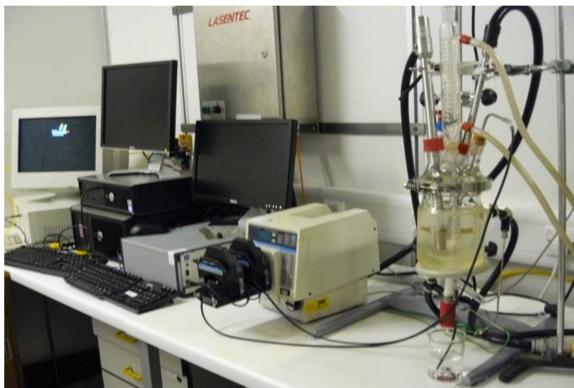
Figure 3.5. Picture of the antisolvent crystallization rig set-up performed with a peristaltic pump (Loughborough University)
