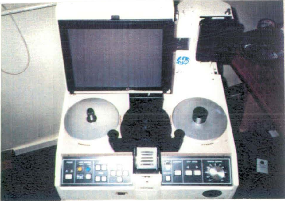
Figure 3.5a Anterior view of CAP35B Cine Projector (International General Electric Company) showing loading spools and controls.
