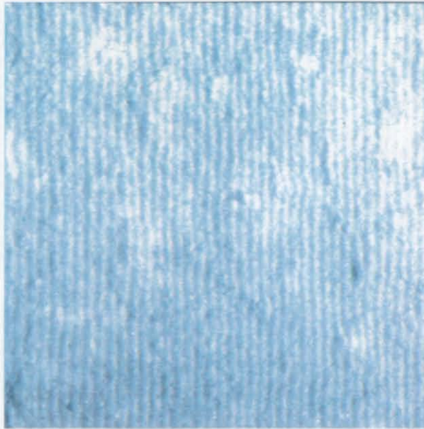
Figure 5.29. Contour fringes on a marble surface eroded by 200 years exposure to natural weathering on the Duomo of Milan.
