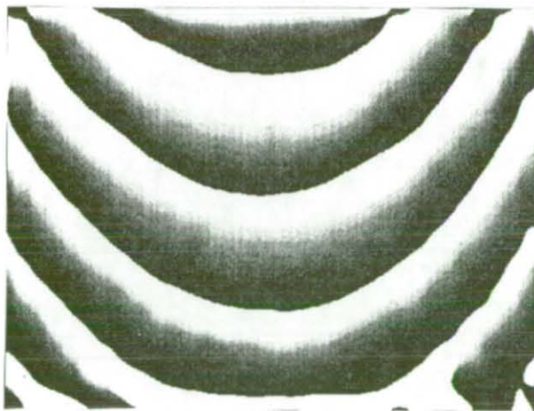
Figure 3.7. a) Endoscopic fringes obtained by holographic inspection with optical fibres. White light reconstruction. b) Power spectrum. c) Phase diagram modulo 2\pi .
