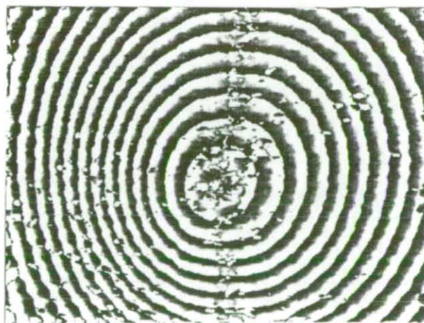
Figure 3.11. a) Circular fringes of an ESPI interferogram. b) Power spectrum. c) Phase diagram.
