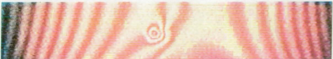
Figure 4.11. Fringe pattern of specimens with different levels of impact energy (A series).
