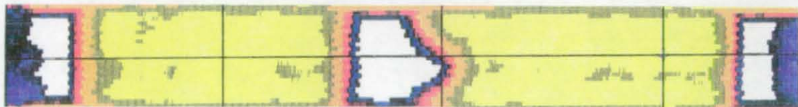
Figure 4.19. Ultrasonic examination of specimens with different levels of impact energy (B and C series).
