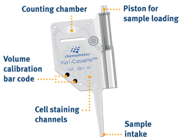
Figure 17. Image of a Vial-Cassette™ from Chemometec detailing the different components of the cassette. Image sourced from NC3000™ product brochure 227
