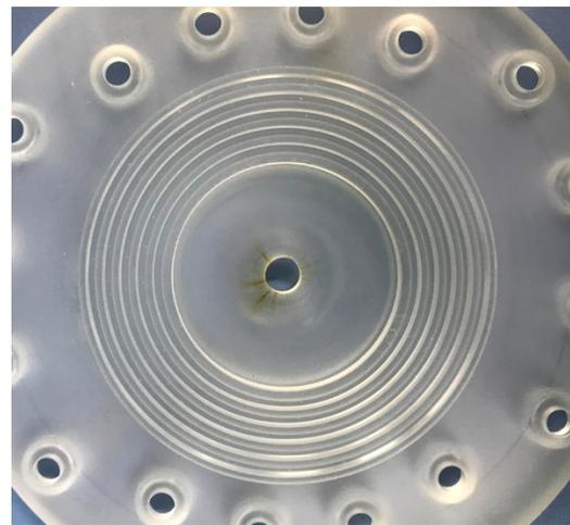
**Fig. 10.** Photo of a plate insulator after 100,000 shots test using the main electrode with sharp edge.
