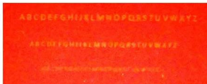
Figure 1 – Letters in Arial font sizes 6 – 4 printed in 0.4 mM alanine and developed using DFO, shown photographed under green light excitation (490-560 nm) with an OG590 camera filter.
