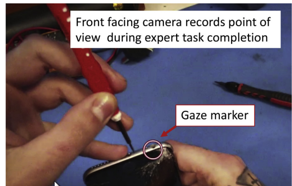
Fig. 4. Eye tracking recording showing point of view of the expert completing task steps (explicit knowledge) and the focus of their visual attention via the gaze marker (tacit knowledge).
