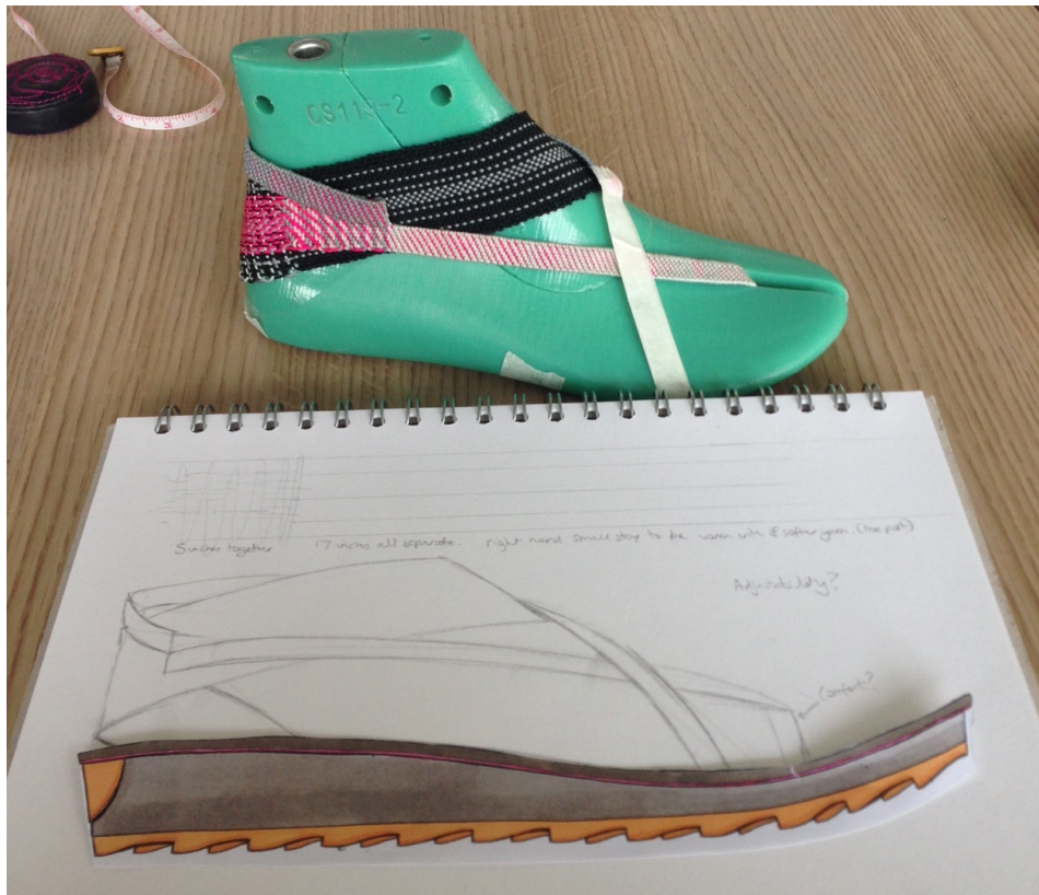
Figure 5: An example of 2D/3D approaches to idea generation involving sketching and quick modeling techniques, © Jenny Pinski.
