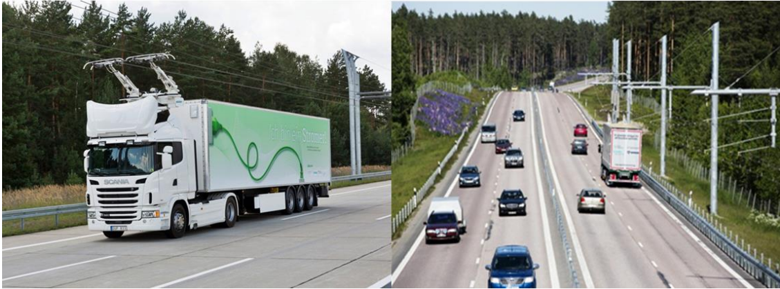
Figure 1.2.4-left, eHighway Innovative electric road freight transport [9]; right, eHighway, Gävle, Sweden [14]
