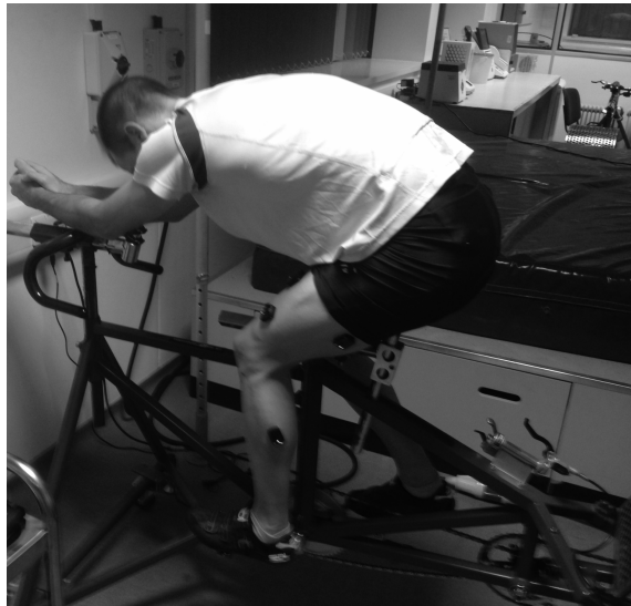
Figure 1: A cyclist performing isometric maximal voluntary contractions using single-joint dynamometry of a knee extensor (left) and isometric cycling (right)
