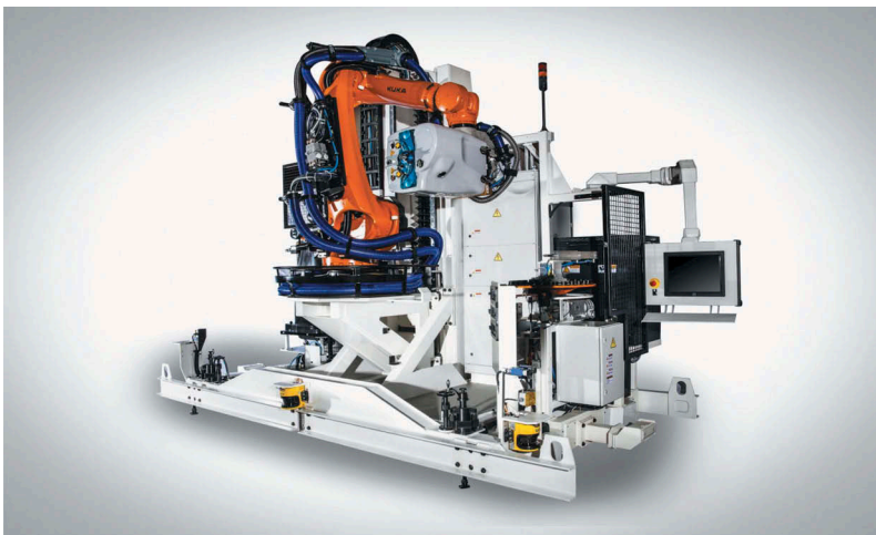
Figure 1. Mobile robotic platform and multifunctional robotic end effector are used for drilling and fastening aircraft wing assemblies (Courtesy of KUKA systems aerospace).
