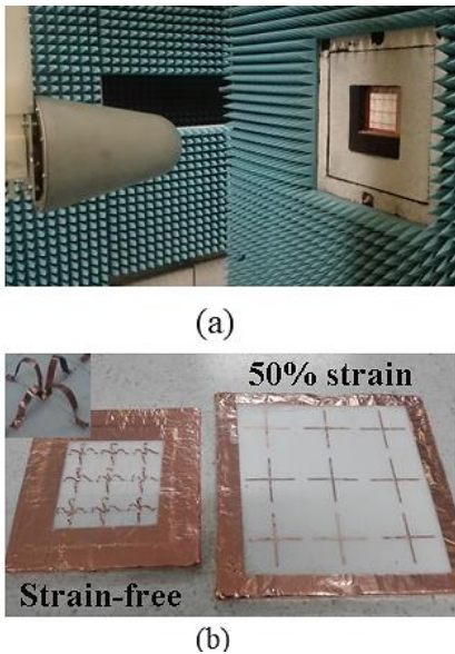
Fig. 2. (a) Experimental set-up, (b) FSS prototypes. The right hand side sample has been undergone 50% strain in its elastomeric substrate and the left hand side sample is strain free.
