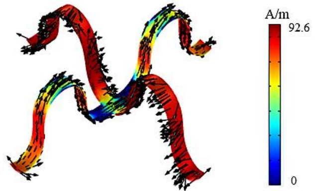
Fig. 4. Surface current (A/m) on the buckled cross-dipole. The currents flow in opposite directions on adjacent vertical arms and have cancelling effect leading the structure to be electrically smaller than the actual physical size.
