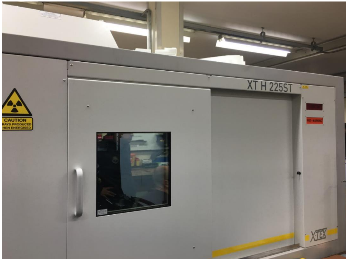
Figure 3.22 Nikon XT H 225 ST industrial CT scanning apparatus used.
