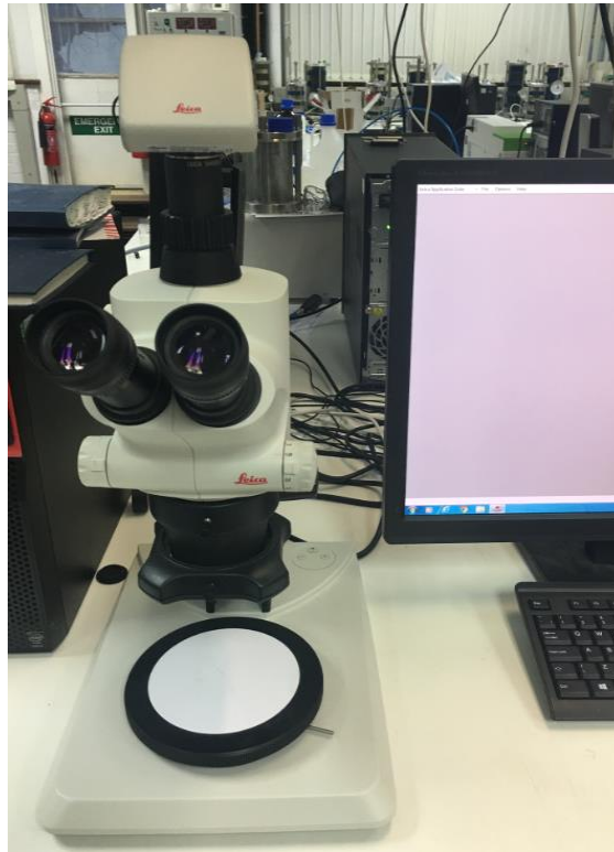
Figure 3.19 The Leica LED2000 optical microscope used to measure and monitor cracks.
