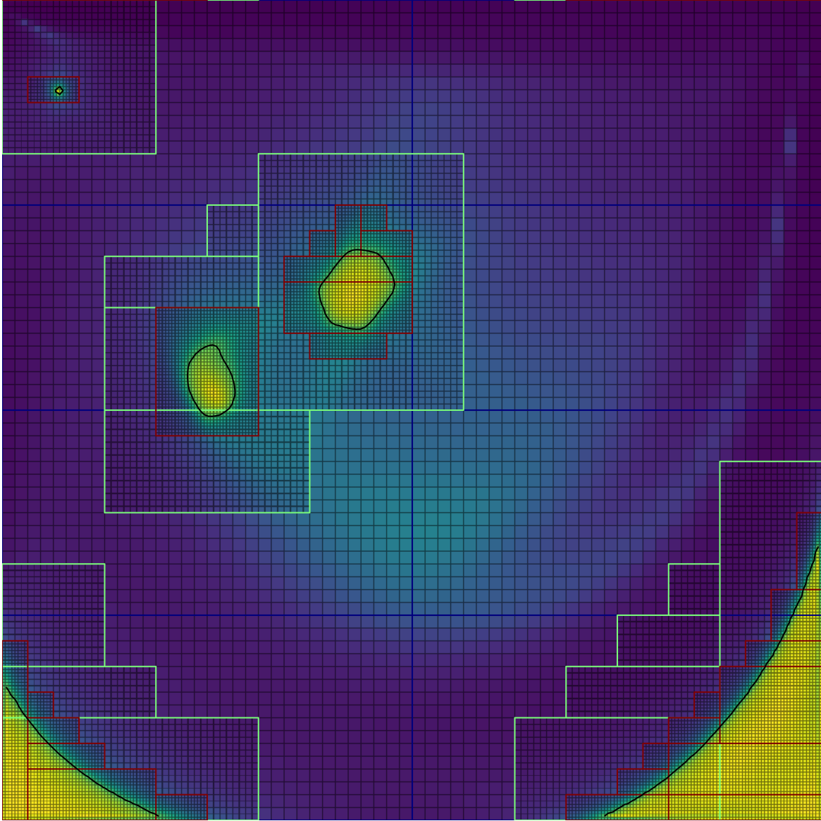
Figure 5.8: Illustration of spatio-temporal adaptive mesh refinement for tracking the development of the yield surface of a Bingham fluid with Re = 1000 and Bi = 1 in the 2D lid-driven cavity. The heatmap shows the magnitude of the stress tensor, which is what the grid refinement criterion is based on. The coarsest grid has cell spacing 1/64 , but the two refinement layers ensure that the effective resolution near the yield surface is 1/256 .
