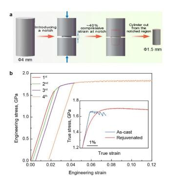
Fig. 1 | Rejuvenation and deformation of an MG. a, A 4-mm-diameter rod of
