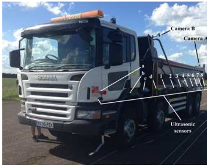
Fig. 2.2 Camera and ultrasonic setup
