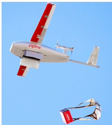
Figure 1.22: The Zipline drone used for delivering a medical cargo upon an order. The drone flies in a 80 km service radius from Zipline distribution centres in Rwanda and Ghana. Image credit, Zipline, flyzipline.com
