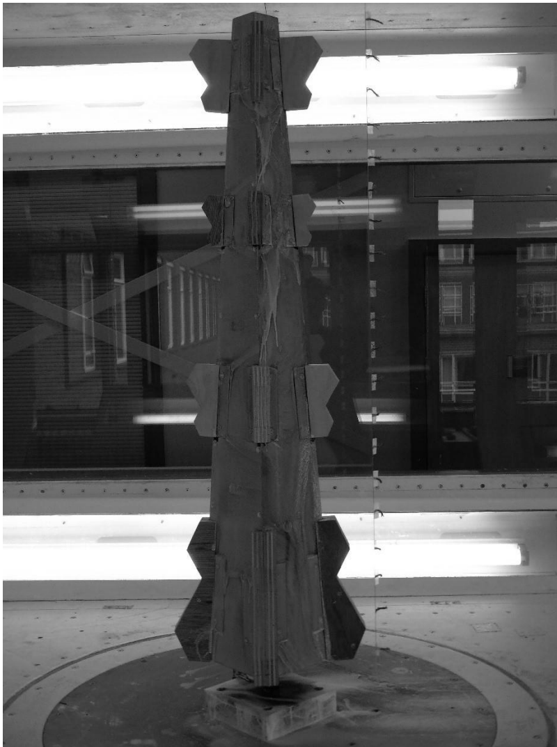
Figure 2 Model pinnacle in the Markham wind tunnel
