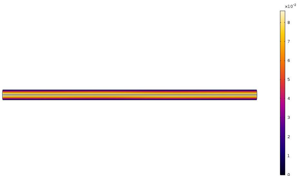
Figure S10: Velocity magnitude (m/s) inside 1.55mm I.D. capillary at sonication residence time of 0.3 s.
