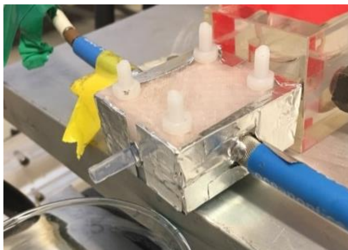
Figure S6: Custom made “Flow through cell” (as in fig. S5) for through the wall absorbance measurements.
