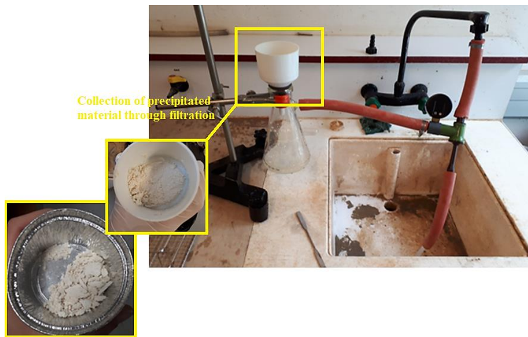
Figure 6.6: Collection of the precipitated material by using a vacuum system that facilitates percolation of the test-tubes content across the filter paper.
