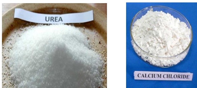
Figure 4.13: Urea powder ( \text{CO}(\text{NH}_2)_2 ) and flakes of calcium chloride ( \text{CaCl}_2 ).
