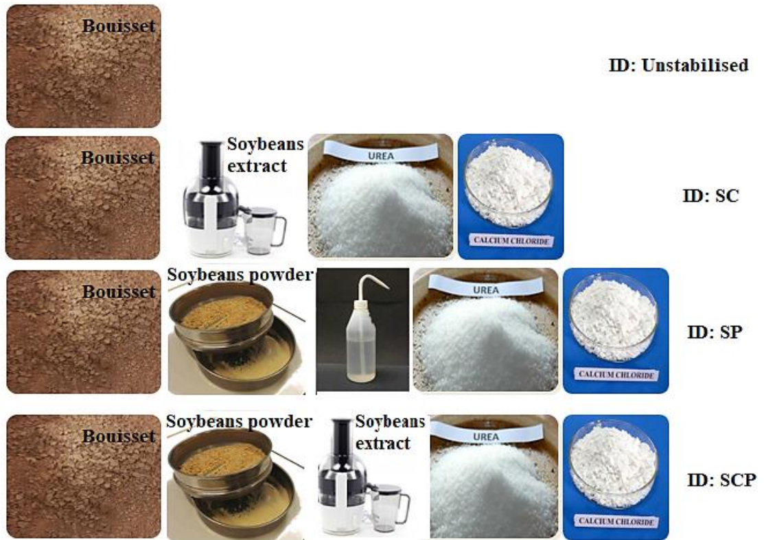
Figure 6.25: Composition of cementing mixture added to the dry earth for SC, SP and SCP stabilisation methods.
