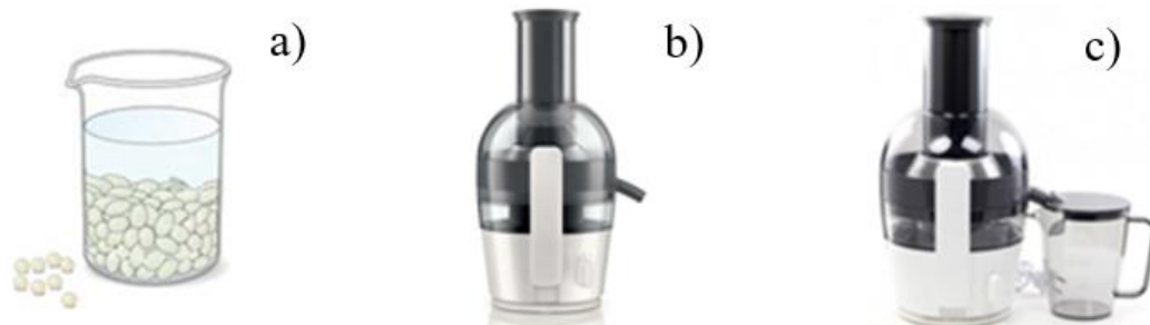
Figure 4.12: Procedure for obtaining the urease enzyme: soybeans are soaked in water (a), soaked soybeans are centrifugated in a blender (b), the crude urease extract is collected (c).
