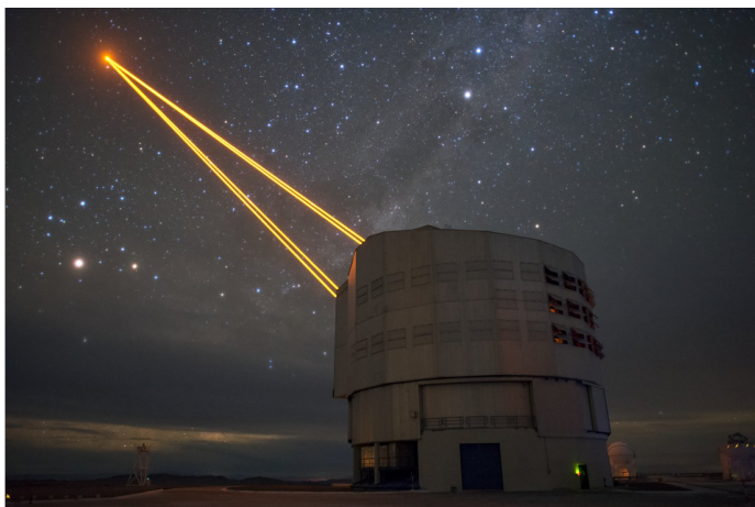
Figure 2.1: Photograph of the 4-LGS system of the AOF on the 8.2 m Yepun telescope at the VLT, Paranal (Kamphues, 2016).
