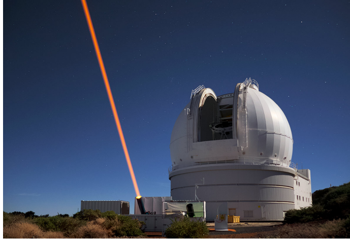
Figure 2.18: Photograph of the sodium LGS used by CANARY on the 4.2m WHT, La Palma (Bardou, 2018).
