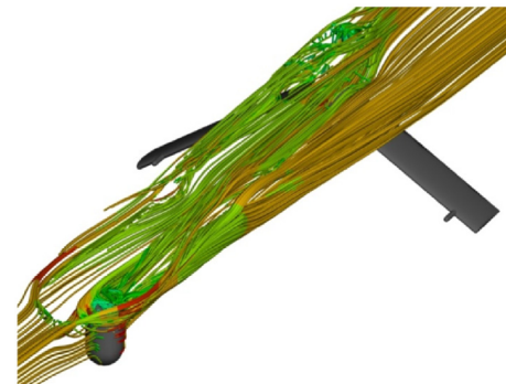
(b) Streamlines on modified geometry (flow spread indicates blanking phenomenon)
