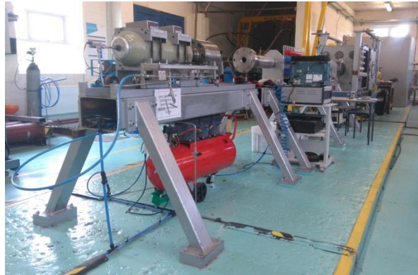
Figure 3.1 Image of the 50 mm bore single stage gas gun at Cranfield University.
