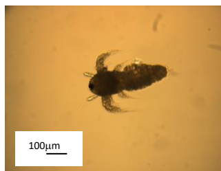
Figure 7.6 Hatched nauplius after shock loading at 0.78 GPa.
