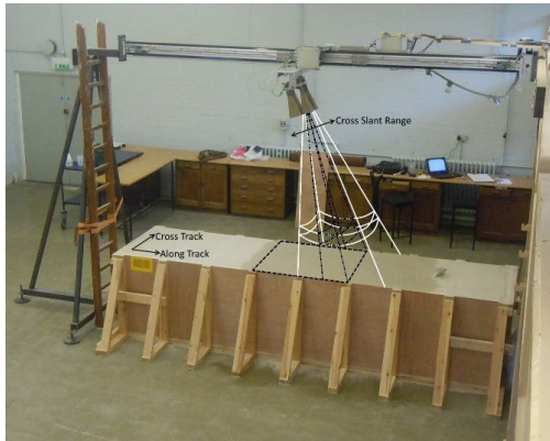
Fig. 1. View of the soil trough and linear scanner with the C-band antennas attached. Note that this photograph was taken while a different experiment was being performed, and hence the wetted area and reference trihedral deployment are different to the situation in this study. Dashed square on trough surface shows area actually wetted during this study. Solid white lines represent the real antenna beam pattern and resolution cell, and dotted-dashed black lines indicate the beam pattern and resolution cell obtained using TP. Coordinate notation as used in text.
