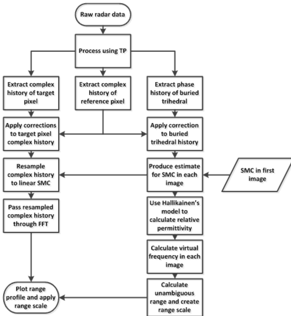
Figure 3.17: Flowchart of the implemented VB-SAR processing function
