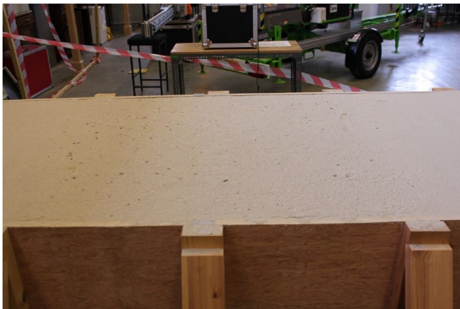
Figure 5.3: 1m x 1m area containing gravel mixture. Trihedral buried 26.5 cm below surface in roughly the centre of the gravel area
