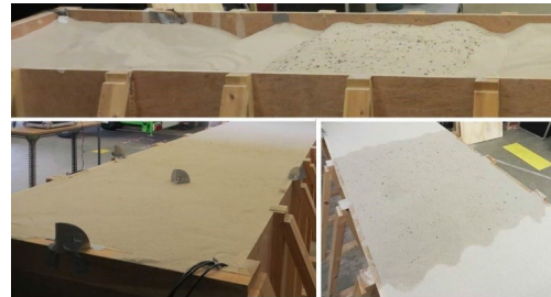
Fig. 3. (Top) Preparation of the soil target. (Bottom right) Wetted 1 m \times 1 m area at the location of the gravel-soil mixture. (Bottom left) Positioning of the reference trihedrals. Darkening of soil surface in vicinity of surface reference trihedrals is caused by shadow.
