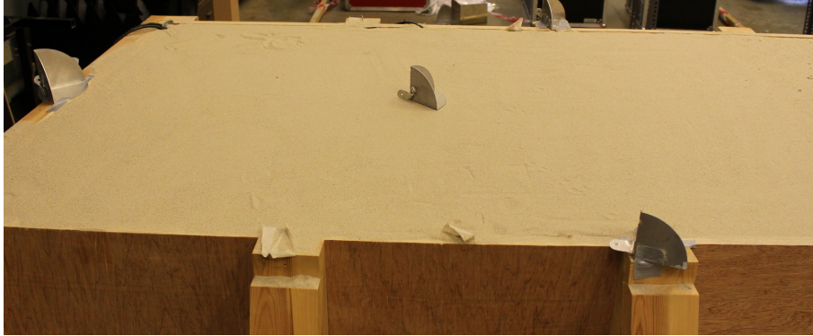
Figure 5.4: Arrangement of reference trihedrals
