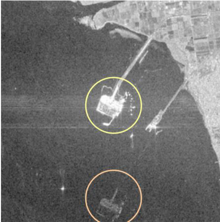
Figure 3.8: Radarsat-2 view of a coastline. "Ghost" image in orange circle is a duplicate of the real feature in the yellow circle [50]
