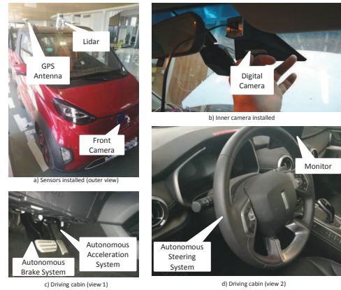
Fig. 7: Experimental setup: Sensors and Systems
