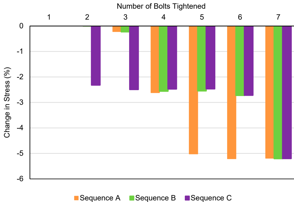
Figure 9. Comparison of bolt Fp using three different tightening sequences.
