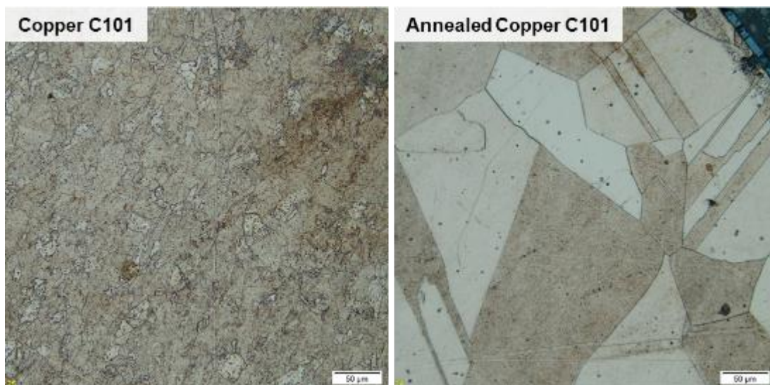
Figure 5.3 Microstructure of Copper C101 before and after annealing.
