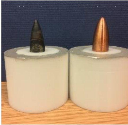
(a) Inserted unjacketed and jacketed cores in 50 mm acetal sabot.
