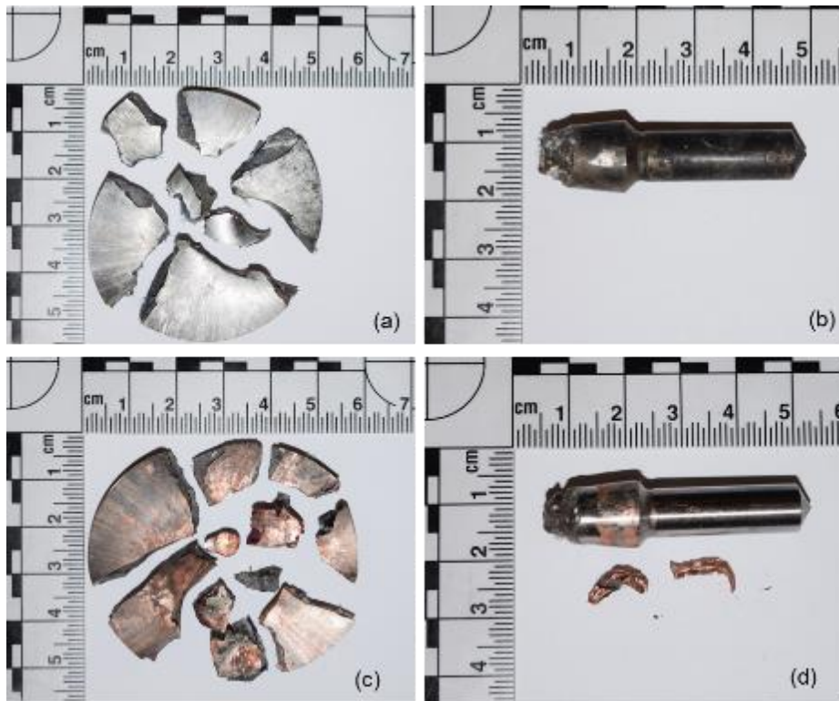
Figure 5.14 Recovered impactors (5-mm thick Armox Advance) and En8 steel cores: (a) and (b) un-jacketed core shots and; (c) and (d) jacketed core shots from Table 5.4.
