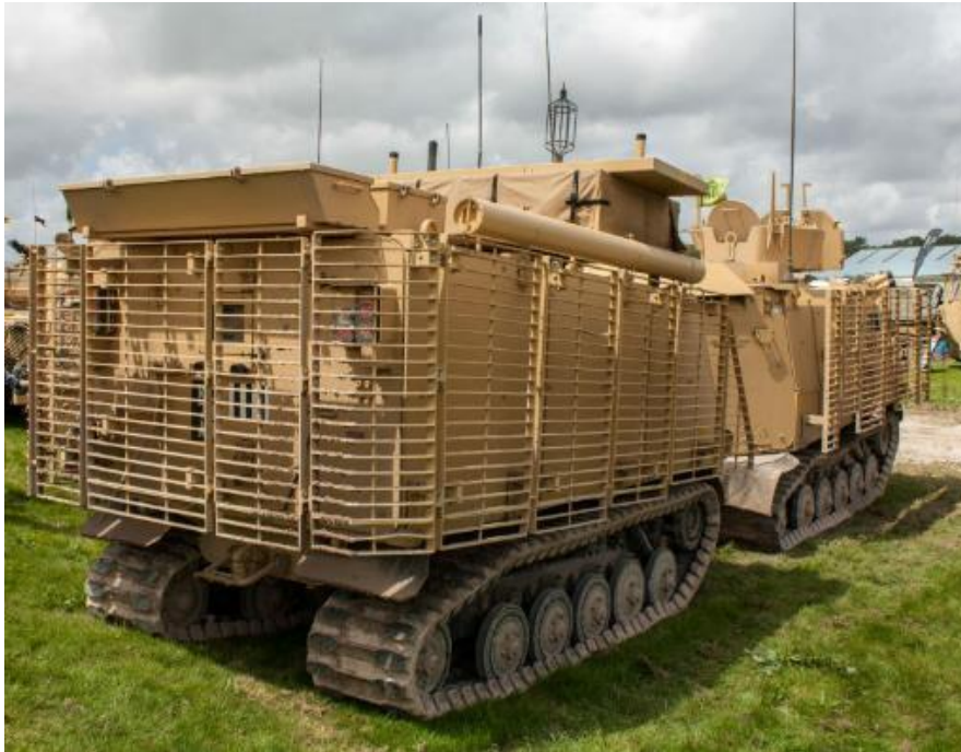
Figure 1.11 Slat armours installed to protect main armour plates (30).
