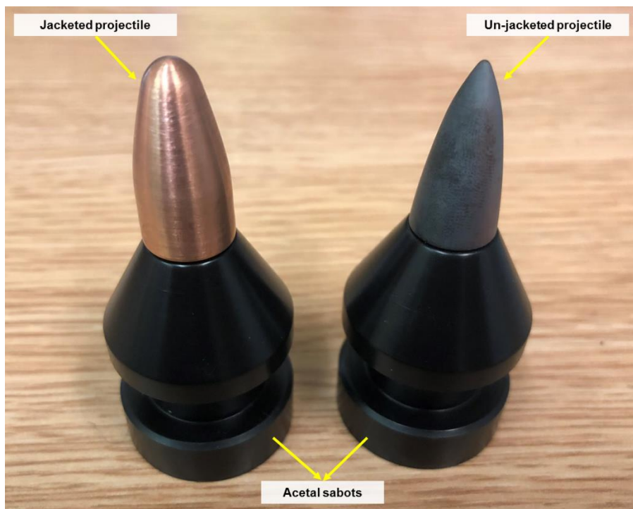
Figure 3.3 Jacketed and un-jacketed projectiles embedded in 30-mm diameter sabot.
