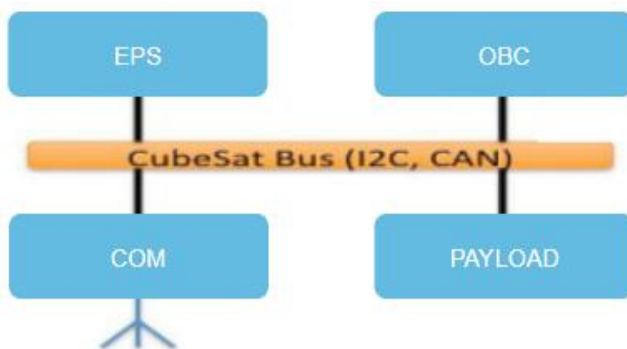
Figura 4.37. Comunicación I2C (Inter Integrated Circuits), CAN (Controller Area Network) [109].
