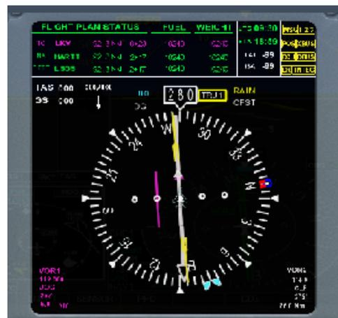
**Gambar 17 B** Instrumen HSI Simulator VOR CLP
