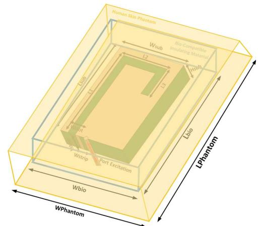
Fig.2 (a) Dimensions of proposed PIFA antenna (b) PIFA design enclosed in bio-compatible insulator and human skin phantom with relevant dimensions.
