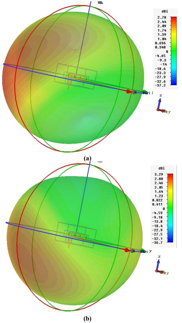
Fig.4 3D radiation plot (a) Directivity at 1.4 GHz (b) Directivity at 2.45 GHz
