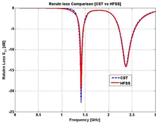
Fig.3 Dual-band return loss  $S_{11}$  of proposed PIFA antenna with comparison done between CST and HFSS
