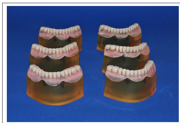
Figure 5. Appearance of finished prostheses with mimic mucosa before occlusal loading on photoelastic models. Prostheses were shaped to clearly view the stress lines around the implants during the photographing of the photoelastic models.
