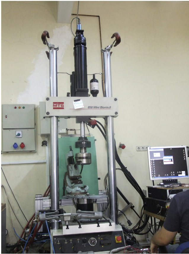
Fig. 4. The MTS 858 Mini Bionix 2-in. universal dynamic test system for measuring load, displacement, and angulation.
