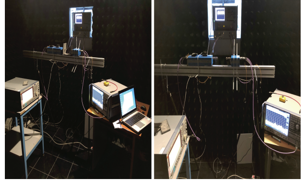
Fig. 1. Two perspectives for the measurement setup in anechoic chamber. LOS conditions are guaranteed by isolating measurement setup and employing anechoic chamber.
